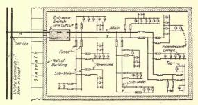
Fig. 146.—An interior distribution "tree" circuit.
